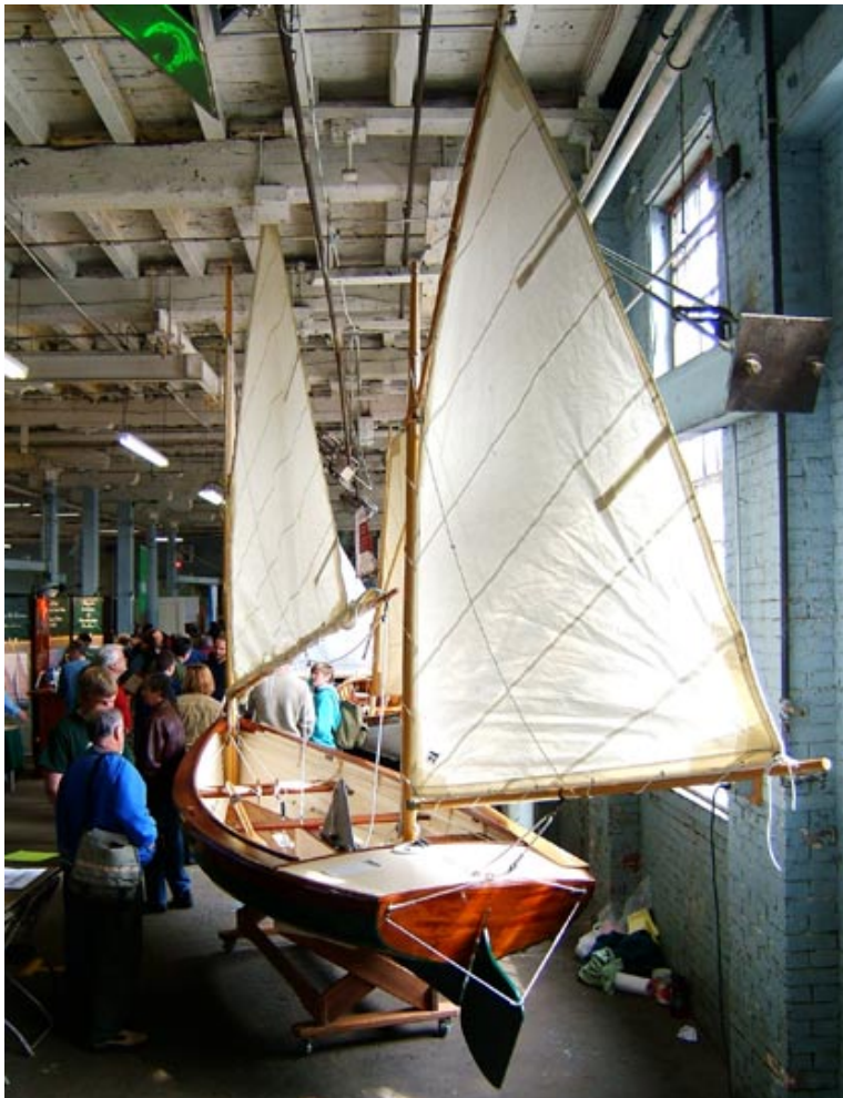
One of the Coquinas on display built of glued lapstrake plywood by Schleiff Boatworks.
