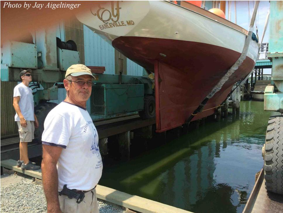
During the haul out, I decided to repack the propeller shaft stuffing box, a necessary evil to minimize water coming into ELF. The shaft couplers were installed with iron bolts and were rusted into new shapes. It took fifteen (15) hours in the small bilge area to cut away and pound out those bolts. When the last bolt was driven out, the engine fell to starboard a bit. (Not a good thing!)
